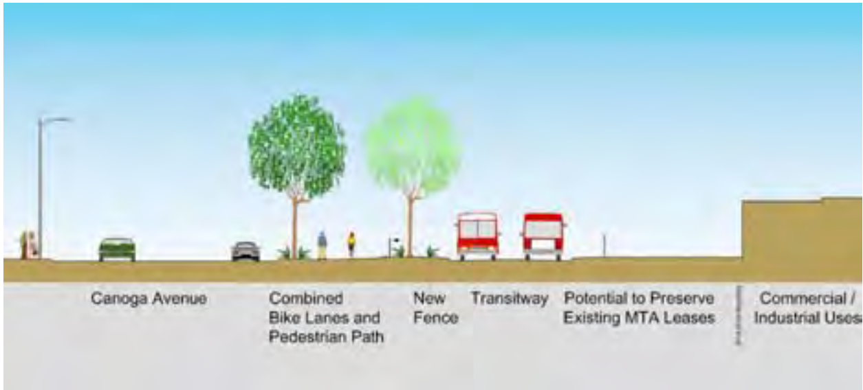
Figure 4-27. Typical Section of Transitway where adjacent to Commercial/Industrial Property
