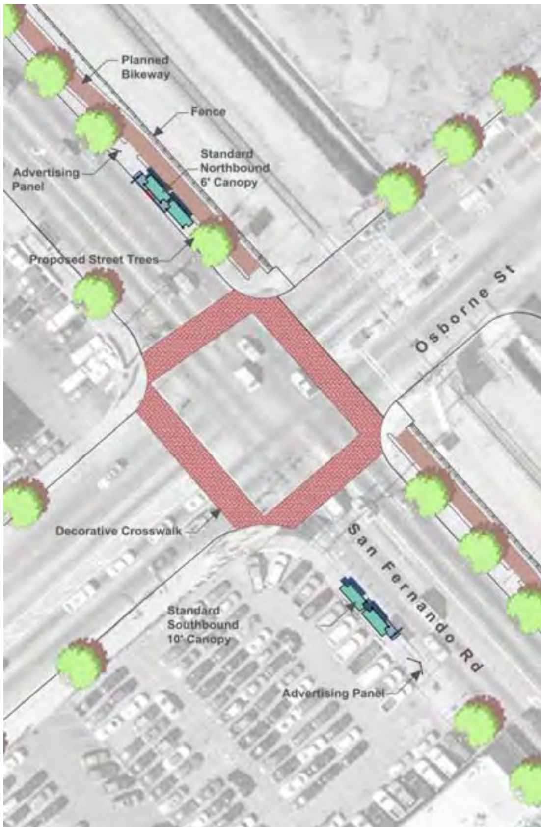
Figure 4-42. Site Plan of On-Street Station along San Fernando Road at Osborne Street
