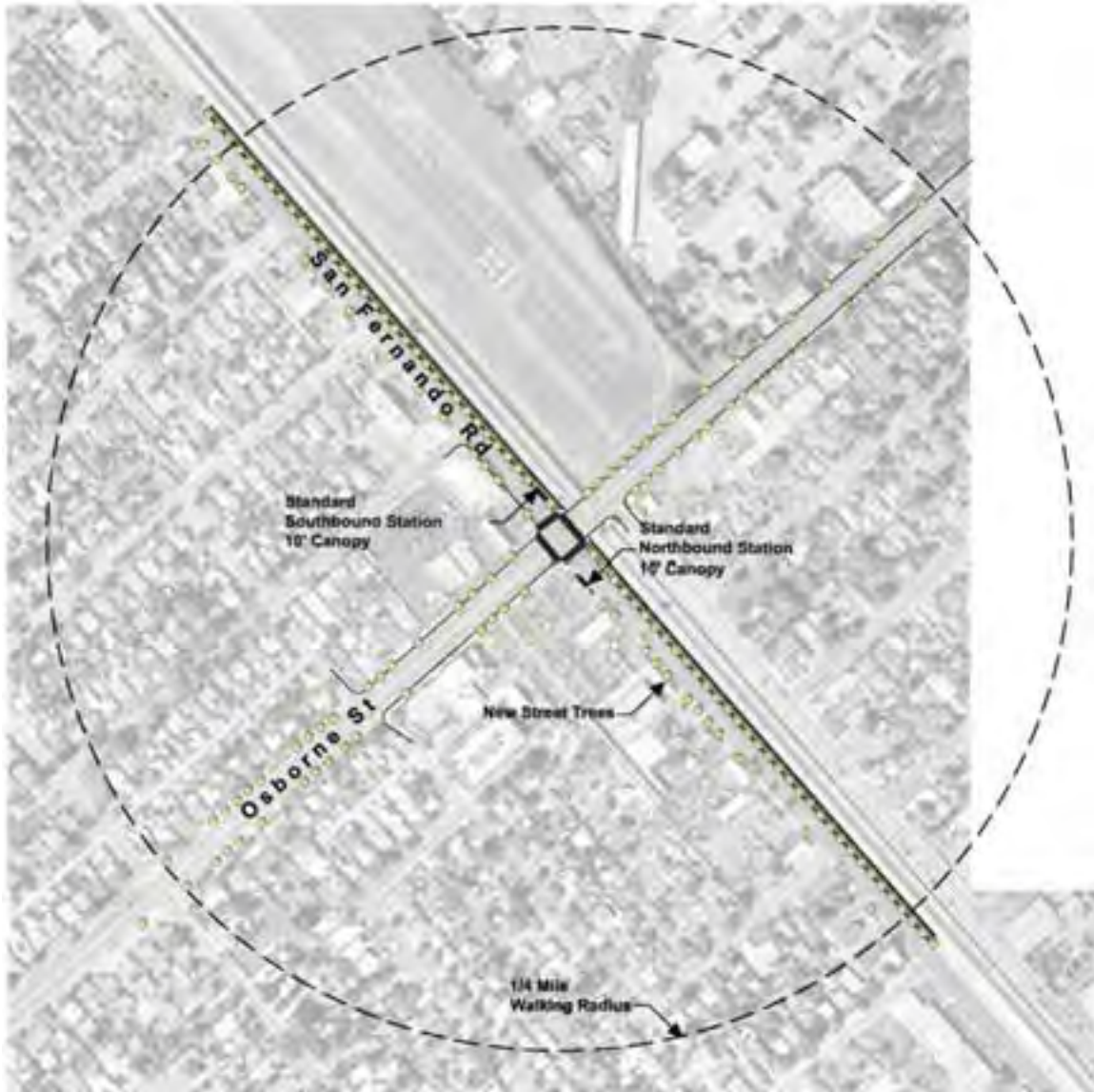
Figure 4-23. Typical Plan of Tree Planting Within ¼ Mile of Station (San Fernando / Osborne Station)
