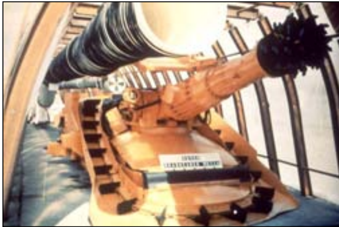
Figure 4-8 Roadheader for Tunnel Mining
