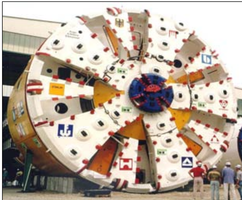
Figure 4-4 Slurry Face TBM used for the 4th Tube, Elbe River Tunnel, Hamburg, Germany
