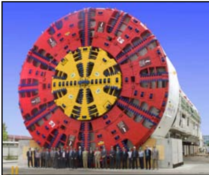
Figure ES-2 Tunnel Boring Machine – Madrid, Spain
