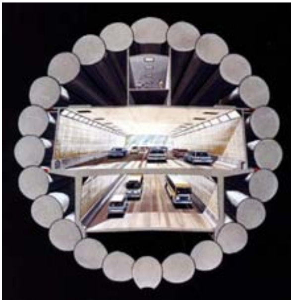
Figure 2-5 Traditional Rendering of Mt. Baker Ridge Tunnel Showing Stacked Drift Construction Concept, Bike Lane at Tunnel Crown
